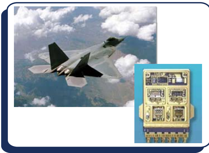
Figure 4-1 Transmit/Receive Module of a Phased Array Radar
