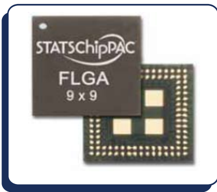
Figure 2-1: Typical LGA package with the central pads shown
