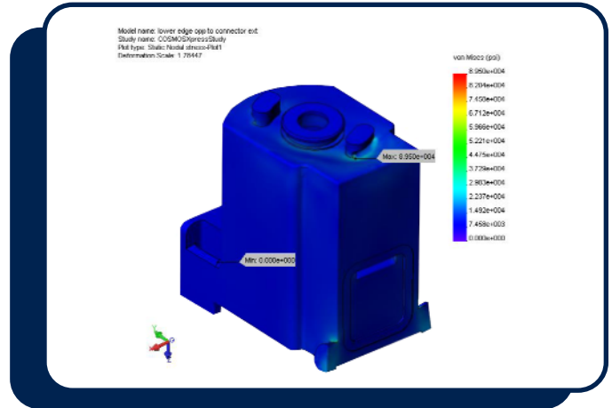
Figure 4-3 – Stress analysis of battery model in Algor
