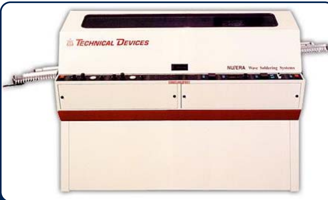
Figure 5-1 – Technical Devices Nu/Era Wave Soldering System
