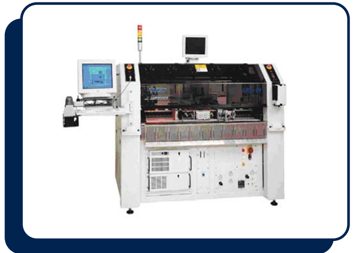
Figure 3-4 – Die Attachment Machine capable of any of the three attachment schemes discussed. (Photo Courtesy of Tyco Electronics)
