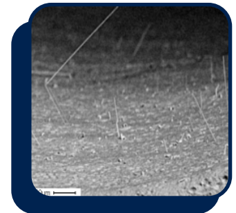
Figure 4-3 - Tin whiskers on an immersion tin plated circuit board, 30 months after plating
