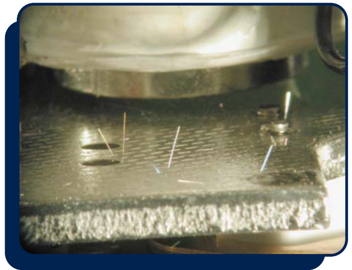
Figure 4-1 - Tin whiskers on a tin plated relay component Courtesy of NASA
