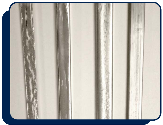
Figure 2-1 - From left to right the alloys are: SnCu, SnCuNi, SnAgCuSb and SnPb
