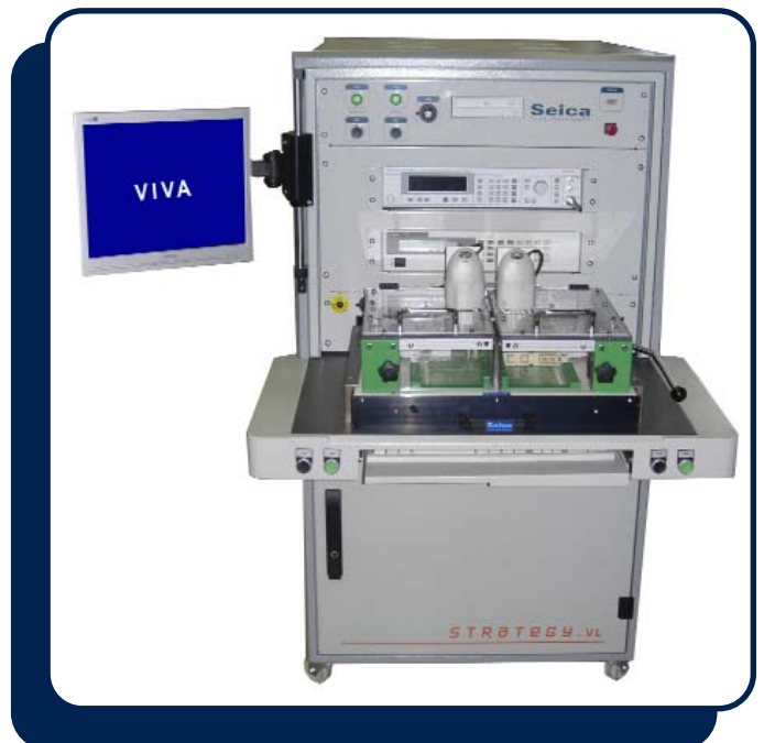
Figure 6-1 – SEICA ATE system
