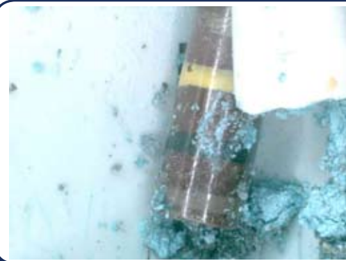
Figure 3. Photo of corroded resistor from a field failure
