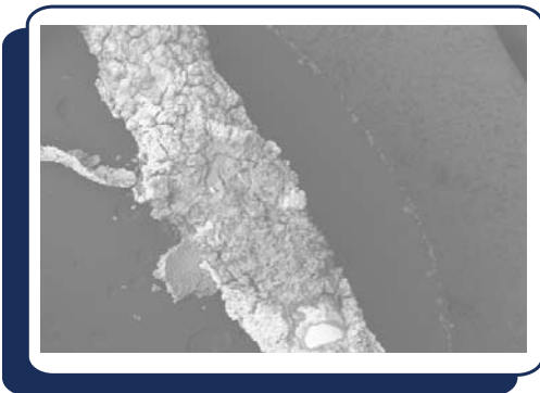
Figure 5. SEM imaging and EDS analysis of the failed resistor leads.
