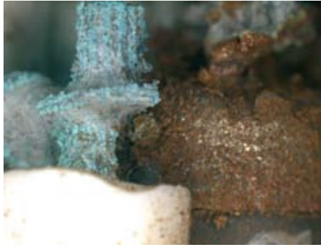
Figure 2. Optical Microscope images and SEM/EDS analysis of corrosion points
