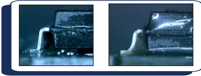
Figure 1. Open and filled lead frames of components from group “J” and “T” (left and right).
