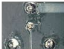
Figure 3-1 Excessive Flux Residues
