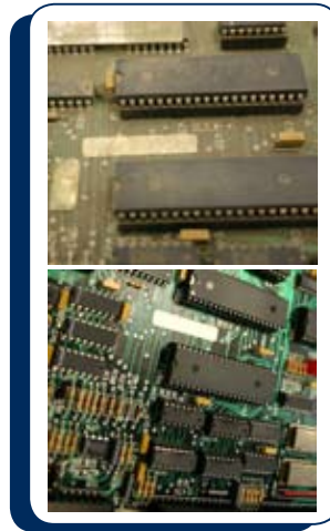
Figure 4-3. Photos of assemblies before (top) and after cleaning (bottom)
