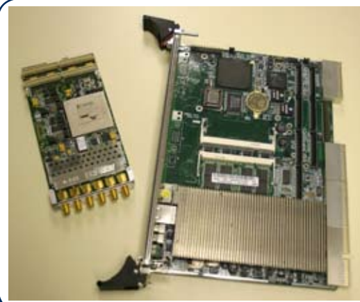
Figure 1-1 Systems conforming to open standards: SDR (left), single board computer (right)
