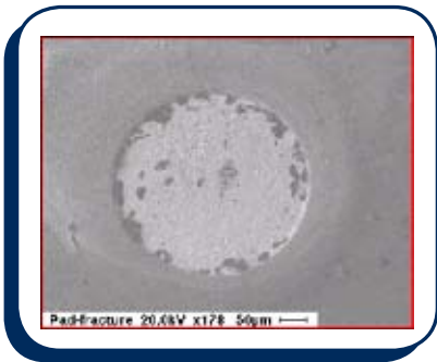
Figure 4-2 SEM image of a BGA ball fracture
