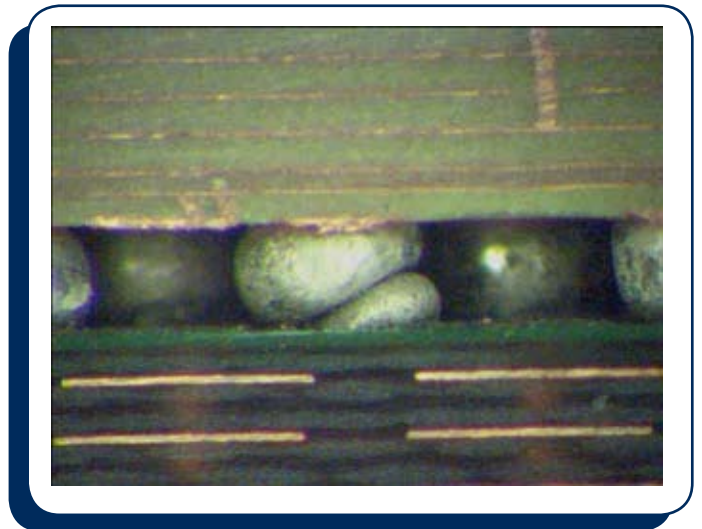
Figure 3-2: A head-on-pillow defect that was verified optically without the aid of mounting and polishing.
