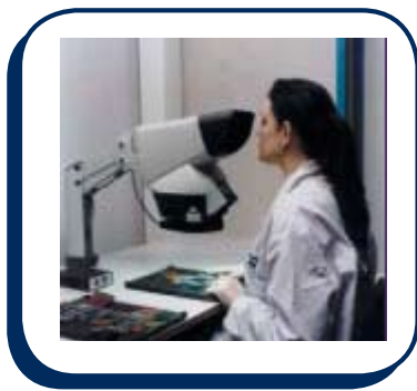
Figure 6-1 UV Inspection of Conformal Coating
