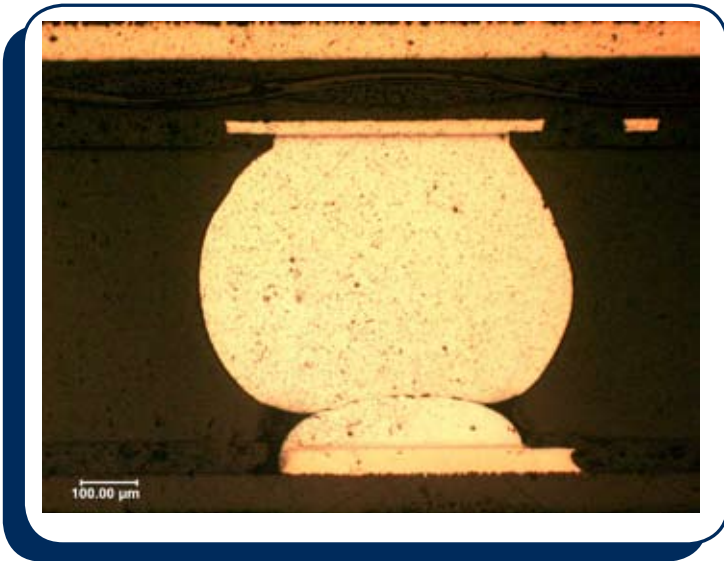
Figure 3-3: Head-on-pillow that required high magnification to be clearly identified
