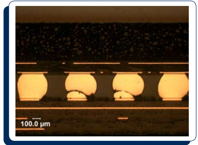
Figure 2-2: TFBGA micro-section of intermittent open locations.
