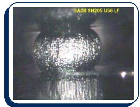
Figure 6-2 non collapsed BGA
