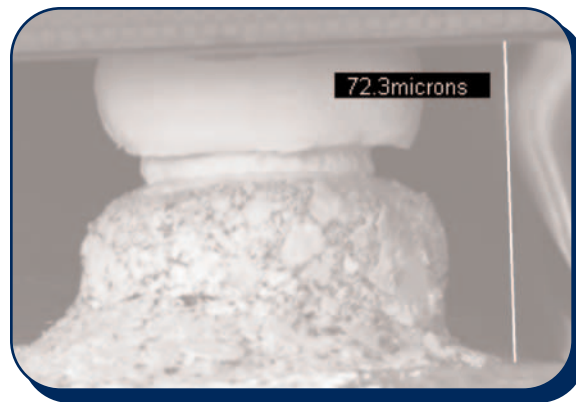
Figure 1-3: Double Stud Bump Attached with Conductive Epoxy
