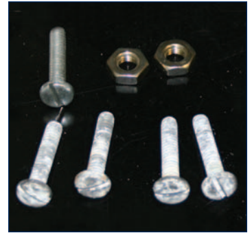
Figure 4-3: The test PCB shown at left, as well as the bolt and nuts in the top portion of the picture on the right, are free from corrosion. The bolts in the lower portion of the photo to the right show the effects of corrosion.
