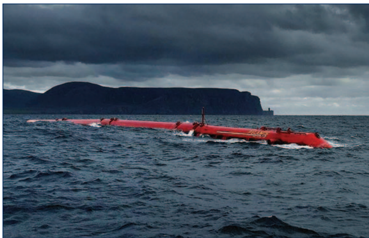
Figure 1-3: Pelamis wave generator used off the north coast of Portugal.
