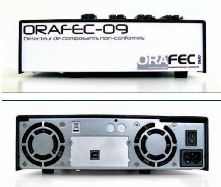
Figure 5-1: ORAFEC Counterfeit Component Detector
