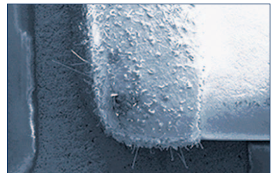
Figure 1-2: Tin whiskers growing from the pure-tin plated terminal of a ceramic component. Courtesy of NASA.
