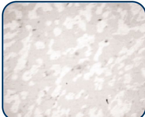
Figure 1. SEM backscatter image of solder microstructure after mild heat treatment.
