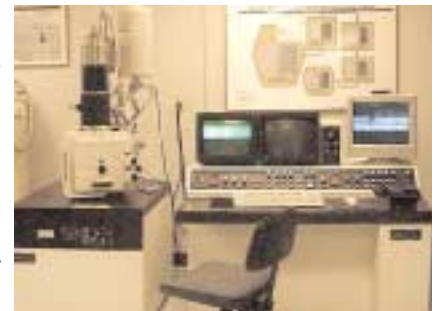
Figure 2. Scanning Electron Microscope (SEM) with Energy Dispersive Spectroscopy (EDS)
