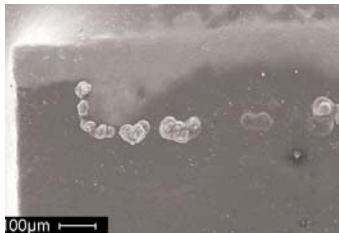
Figure 1. Nodules of corrosion product on failed resistor.
