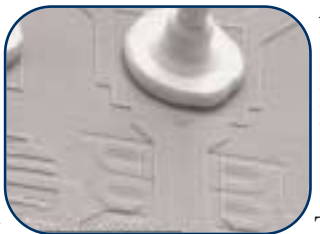
Figure 3. Top down angled SEM image of a ball bond and Ground metallization circuitry
