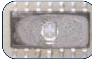
Figure 1. A device after decapsulation showing the die surface
