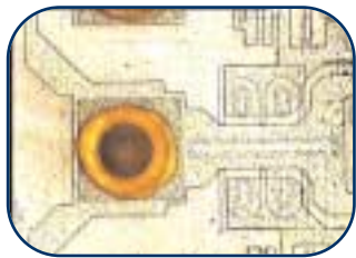
Figure 2. Optical microscopy showing die circuitry and metallization buss at approximately 200X
