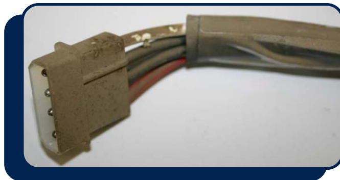
Figure 2-1 – Contaminated connector exposed to hurricane floodwaters.
