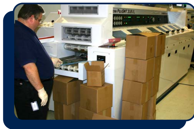
Figure 2-2 – In-line cleaning operation used at the EMPF to recover boards affected by hurricane damage
