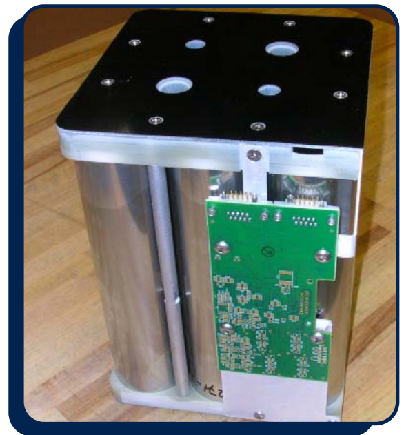
Figure 4-1 – 36V 9 cell module with monitoring electronics
