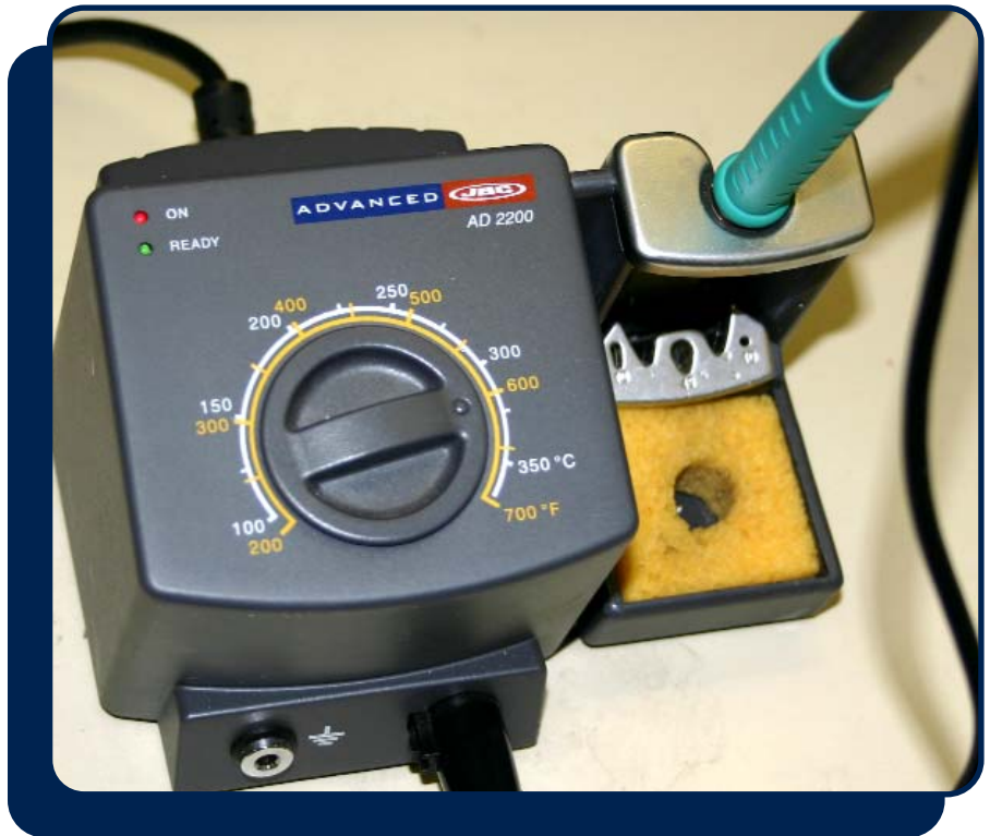
Figure 5-2 – JBC Advanced Series soldering iron
