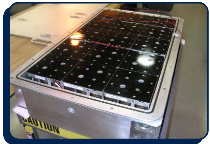
Figure 4-2 – 6061 T6 Aluminum underwater container for modules
