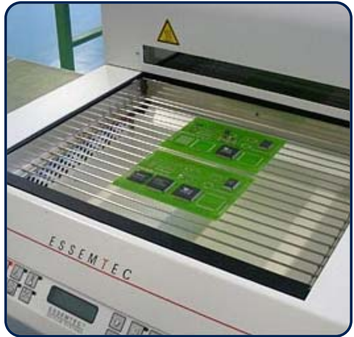
Figure 7-1 – The PCB holder of the ESSEMTEC RO06-Plus
