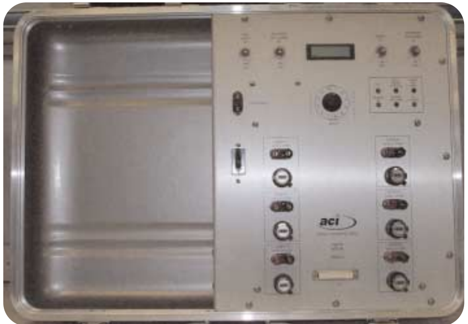
Figure 1: DC-DC converter designed to be powered by a 12-volt battery
